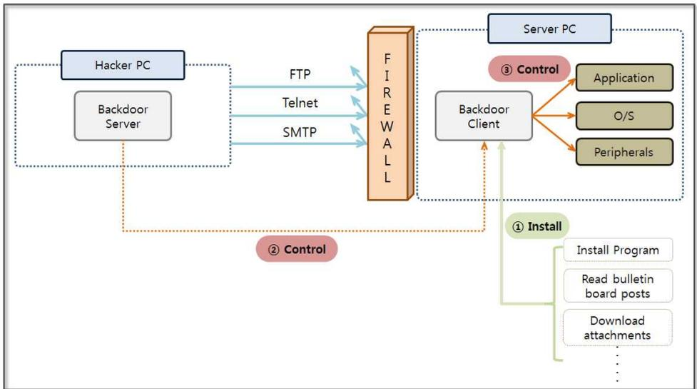
**Figure 5-2 The Basic Concept for a Backdoor**
