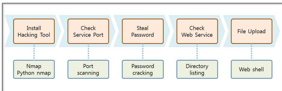
**Figure 4-17 Port Scanning Hacking Procedure**
