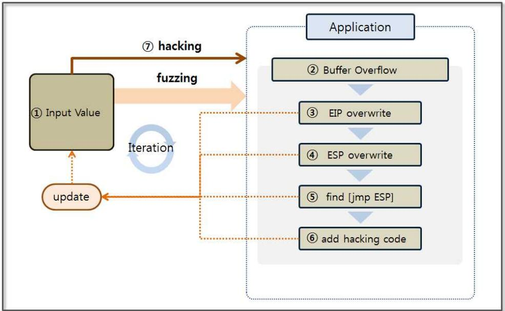
**Figure 5-17 Stack Based Buffer Overflow Basic Concept**
