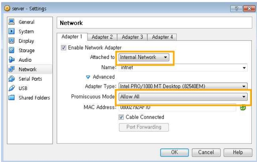
**Figure 3-21 Setting of the Internal Network of Adapter 1**
