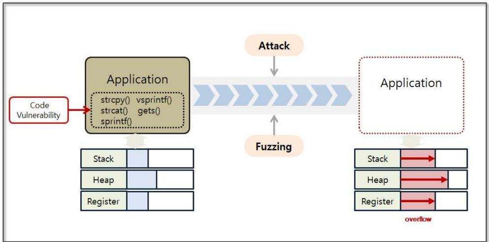
**Figure 5-16 Basic Concept of a Buffer Overflow**
